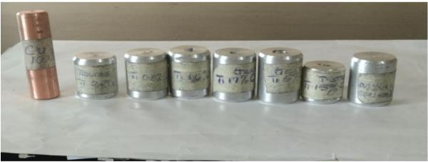
Figure 2: Developed beta phase Titanium copper specimens and copper specimen
