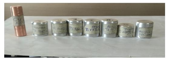
Figure 1: Developed beta phase Titanium copper specimens and copper specimen
